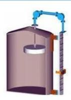
Float and board level indicators are used for fluid level measurements in several industries. The float that is contained within a magnetic level indicator is of course the most important element of the instrument. In fact, its structural design, volume displacement, weight, and buoyancy force are all taken into careful consideration when a float is specified for a particular application.
